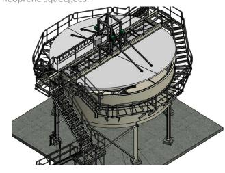
The blades are angled so that sludge is pushed to the centre of the tank, where it can be recirculated or wasted.
