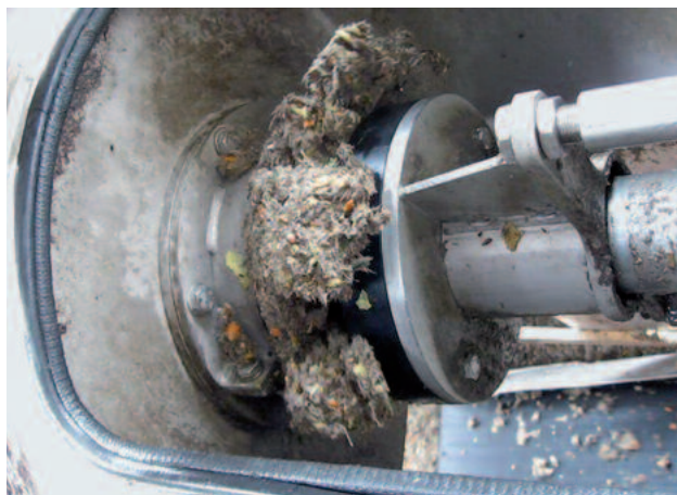
Discharge of the separated compacted material
