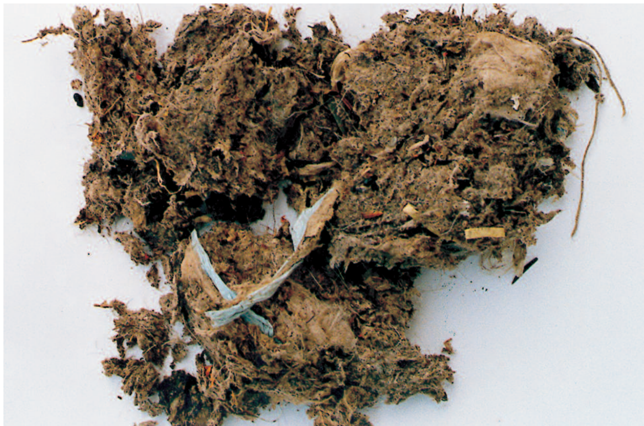
Separated material: paper, wood, plastic, tinfoil, rubber, textiles, etc.
