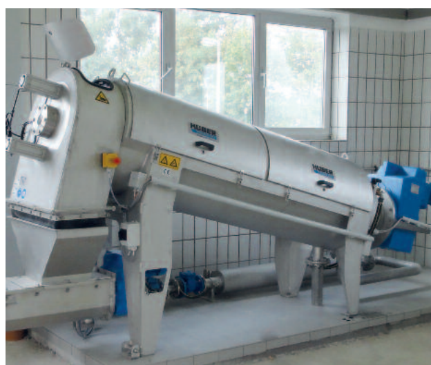
Stationary mounted screw press for 140 kgDS/h
