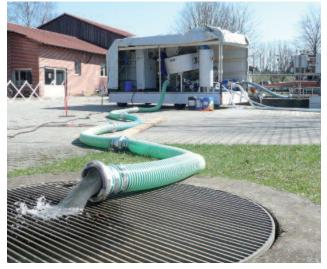
Mobile ROTAMAT<sup>®</sup> Disc Thickener RoS 2S mounted on a car trailer, clear filtrate water runs off in the foreground
