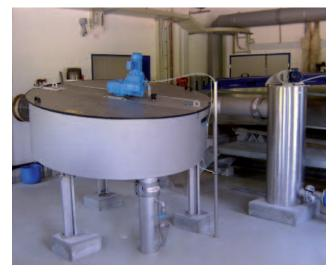
ROTAMAT<sup>®</sup> Disc Thickener RoS 2S size 2 with preceding flocculation reactor
