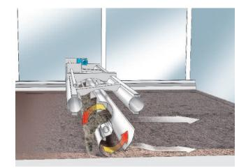
The rotating shovel of the sludge turner takes up sludge and spreads it on the sludge bed; As the turning device gradually travels forward, the entire bed is mixed and restacked
