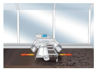
Controlled sludge transport from one place to another as the turner moves with a filled shovel
