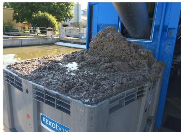
**Fig. 9: Predewatered fine screenings from *HUBER Screenings Wash Press WAP<sup>®</sup> liquid* for digestion [8]**
